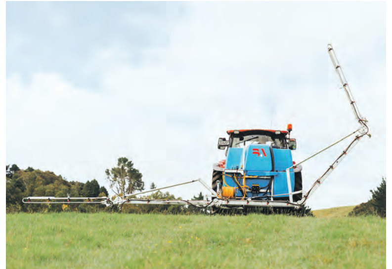
The game-changing LM Linkage Sprayer and M-fold Boom has a full wing lift operated by just two tractor remotes to raise, lower, open or close the boom from the tractor seat.
