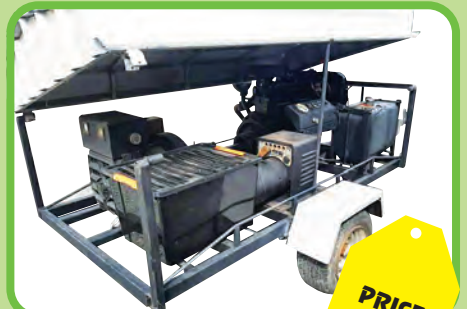
Nissan Industrial 46 horse power engine Welder 250 D.C Generator 10 KVA Single and 3 phase
