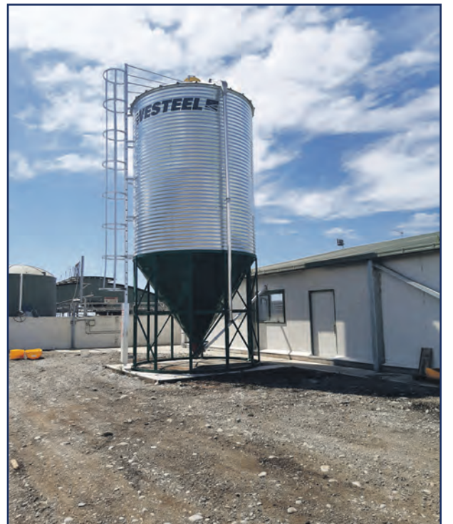
Blend silos, perfect for feeding non-flowing product.
